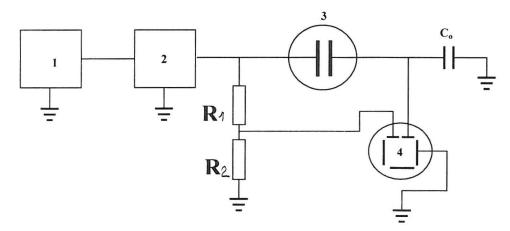
Fig. 2. Electric setup scheme. 1-generator, 2-amplifier, 3-plasma source, 4-oscyloscope.
