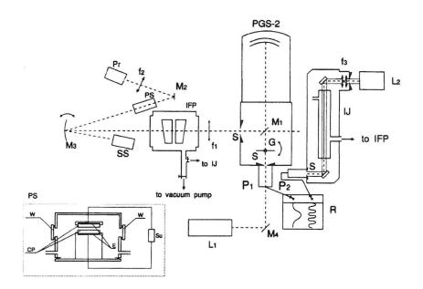
**Fig. 1.** Experimental setup; projector (Pr), lenses (f1, f2, f3), mirrors (M1, M2, M3), lasers (L1, L2), Farby-Perot interferometer (IFP), Jamin interferometer (IJ), grating (G), two-channel recorder (R), slits (S), plasma source (PS), standard source (SS), photomultipliers (P1 or OMA4, P2), spectrograph (PGS-2), windows (W), ceramic plates (CP), electrodes (E), supply (Su).
