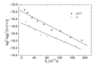
Fig. 5. Boltzmann plot for rotation temperature determination.
