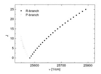
**Fig. 4.** Fortrat parabola for a  $N_2^+$  B<sup>2</sup> $\Sigma_u^+$  - X <sup>2</sup> $\Sigma_g^+$ .
